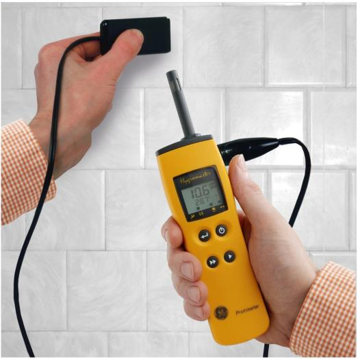
Protimeter Hygromaster measuring surface temperature for condensation readings
