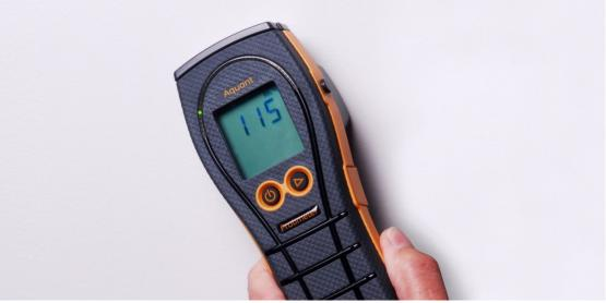
Protimeter Aquant2 taking a non-invasive moisture reading
