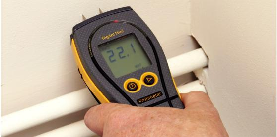
Protimeter Digital Mini taking a surface moisture reading
