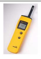
The Hygromaster measures relative humidity and temperature. For flooring applications, it is used in **combination** with a **humidity box** or **humidity sleeves** to measure the equilibrium relative humidity (ERH) of solid floors prior to laying decorative floor coverings. The humidity (and temperature) measurement is made with the removable and replaceable Hygrostick sensor, shown at left plugged into the top of the instrument.
