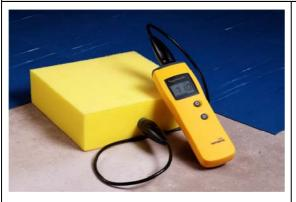
The humidity box is a block of closed cell, high-density foam that is used to isolate a pocket of air at the floor surface from the surrounding environment.
