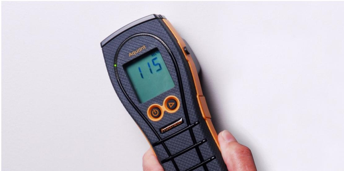
Protimeter Aquant2 taking a non-invasive moisture reading
