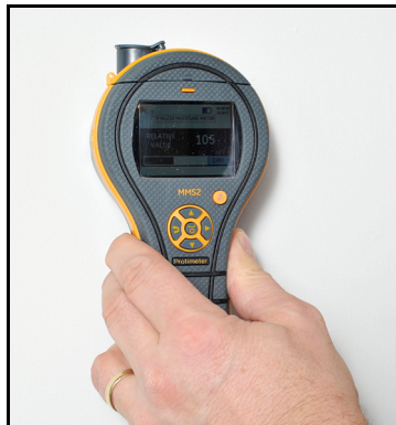
Figure 3: Taking Relative Moisture Readings
