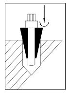
5. Measure the %rh in the hole. This is the ERH value of the floor slab.
