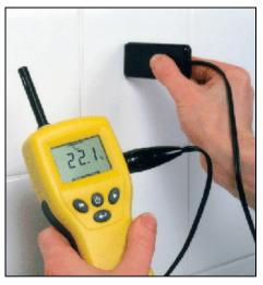
press ► to select *relative humidity* (%rh), *ambient temperature* (TAIR), *dew point temperature* (TDEW), *surface temperature* (Ts) or *temperature difference* (TDIFF) as required. Ts and TDIFF measurements can only be obtained if a
