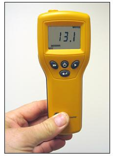
**4.** After about 10 seconds, the display should return to normal and the instrument should read zero when held in free air.
