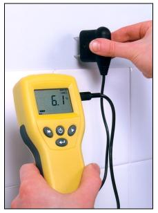
The measured value is displayed and the progress bar indicates whether the material is in a **DRY**, **AT RISK** or **WET** condition, as listed in Table 2 below.
